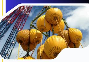
Water filled bags are a unique, proof load testing method for marine, industrial and engineering applications. Working in a defense, oil and gas, shipping and marine markets, we have delivered systems and services to help our clients maintain availability and capability of their assets, in compliance with IMCA standards and LOLER regulations.
